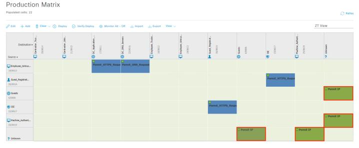
**Note:** Although the Matrix allows all traffic from Unknown IPs to Guest and Machine\_Authenticated SGTs, stateful firewalls will deny any inbound connections to the Guest and Machine\_Authenticated Security Groups. Only return traffic to outbound connections will be permitted by the firewall.
