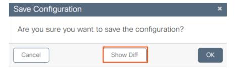
Review the modified running configuration and note that local login configuration may have been removed. It is recommended to verify successful SSH authentication before saving the config to startup.
