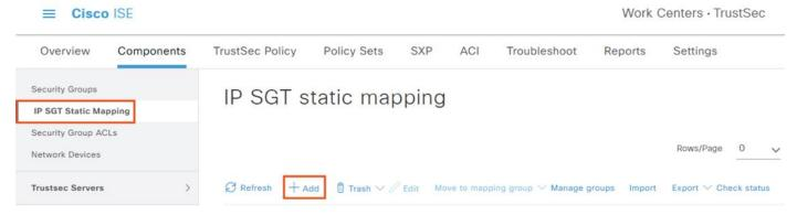
**Step 2.** Specify the IP address(es), leave the radio selection on Map to SGT Individually, select the DC\_Application\_Servers SGT, send the mapping to the DC Application Servers SXP domain, and select TrustSec devices to deploy the mapping to. Click Save.
