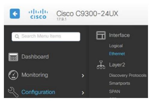
**Step 2.** Click a single interface or select multiple interfaces and click the Multi Port Configuration button (note: Multi Port Configuration will return the selected interfaces to a default configuration and is best used for initial setup). For this example, we will modify the Te1/0/1 interface.
