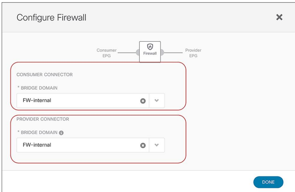
Figure 149. Selected BDs to the consumer and provider connectors for east-west traffic flows (one-arm use case)
