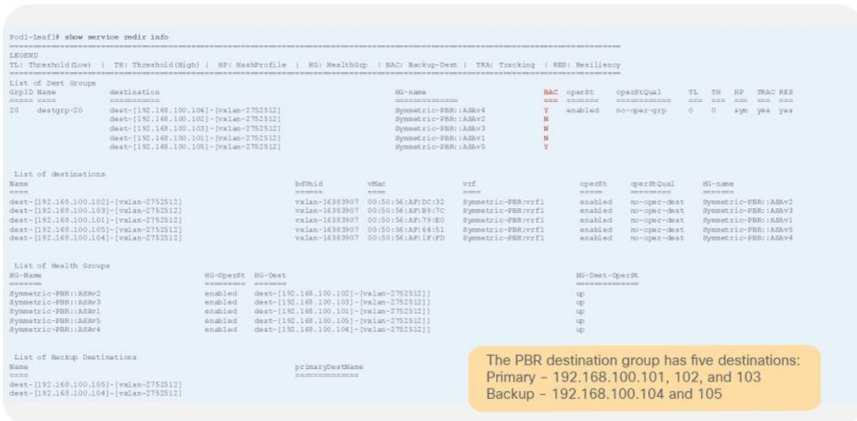
Figure 136. Tracking and backup status on consumer/provider leaf nodes (All PBR destination are UP.)
