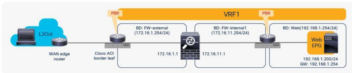
Figure 32. Intra-VRF design (L3Out EPG to Web EPG)
