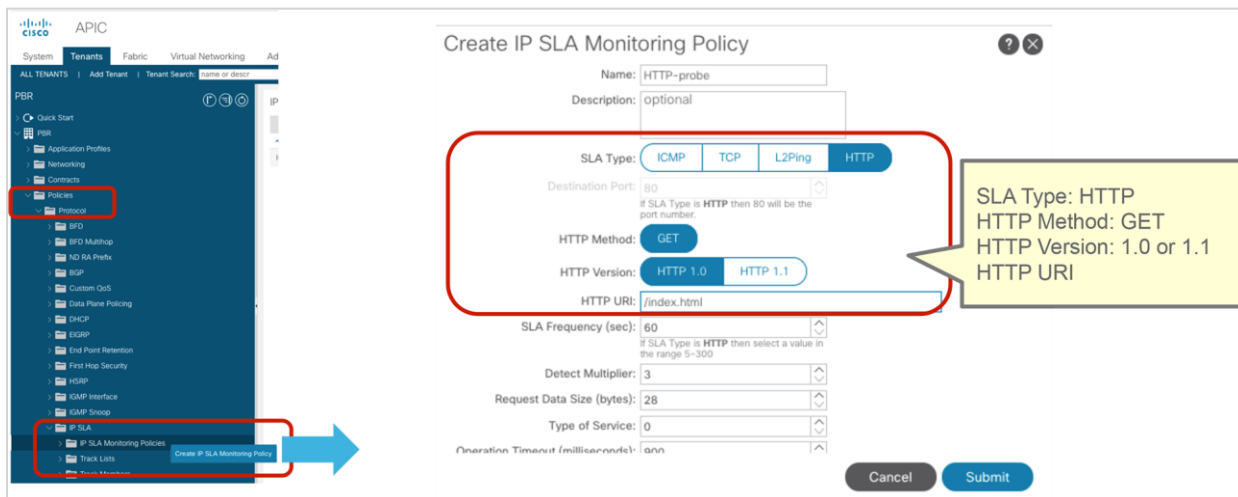
Figure 131. IP SLA monitoring policies (HTTP)
