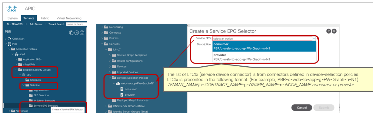
Figure 19. Service EPG selector for ESGs
