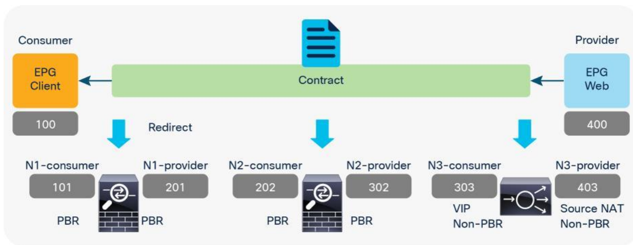
Figure 47. Combination of PBR and non-PBR nodes (Node 3 is Load Balancer with Source NAT.)
