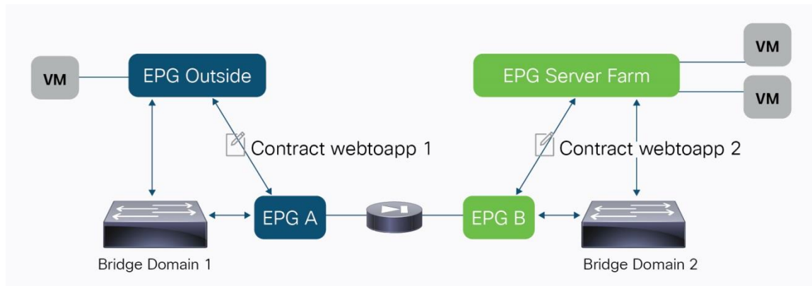
Figure 5. ACI Creates Shadow EPGs and Contracts to Allow Communication with the L4-L7 Device
