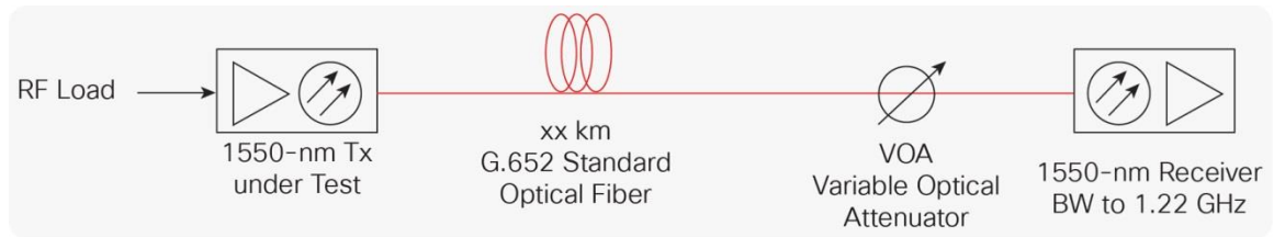
Figure 2. Transmitter Module Test Link Configuration
