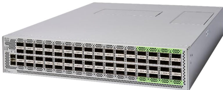
Figure 1. Cisco Nexus 9364C-H1 switch, front view
