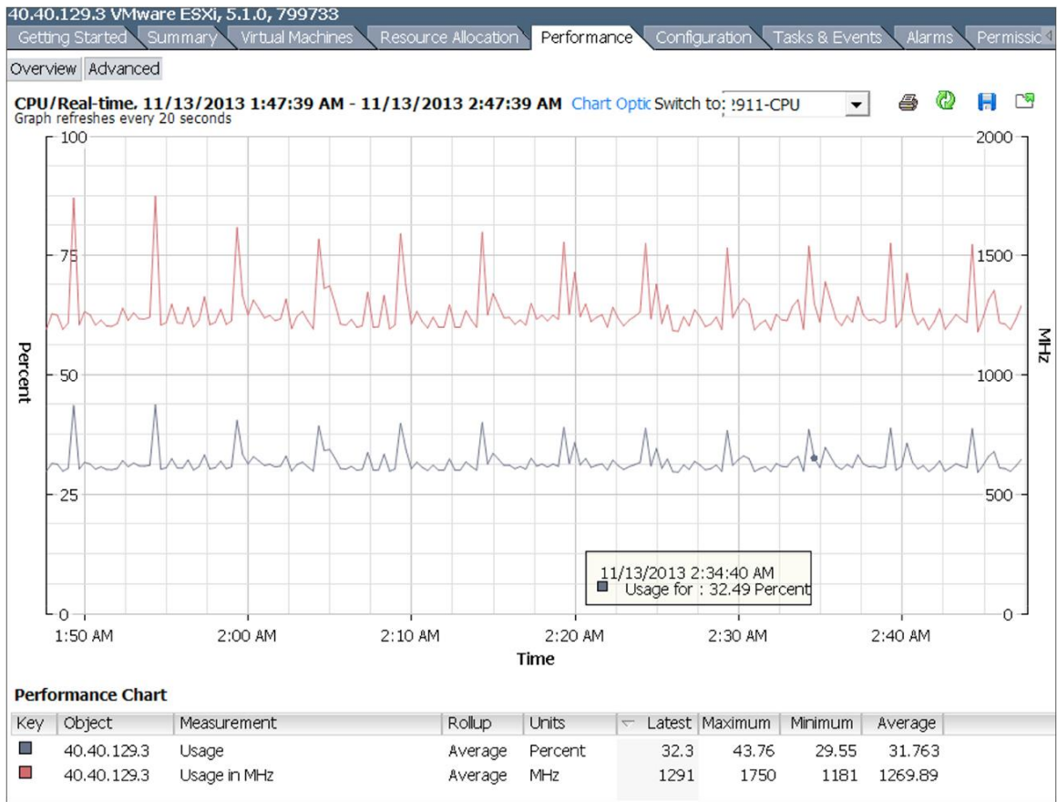
Figure 4. Overall CPU Utilization of the Cisco UCS E140S
