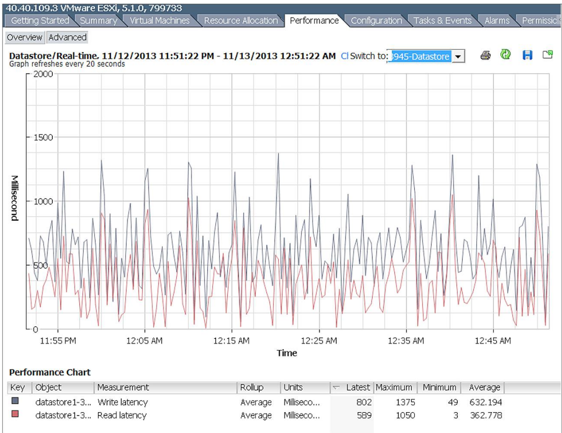
Figure 9. Read and Write Latency of the Cisco UCS E140D
