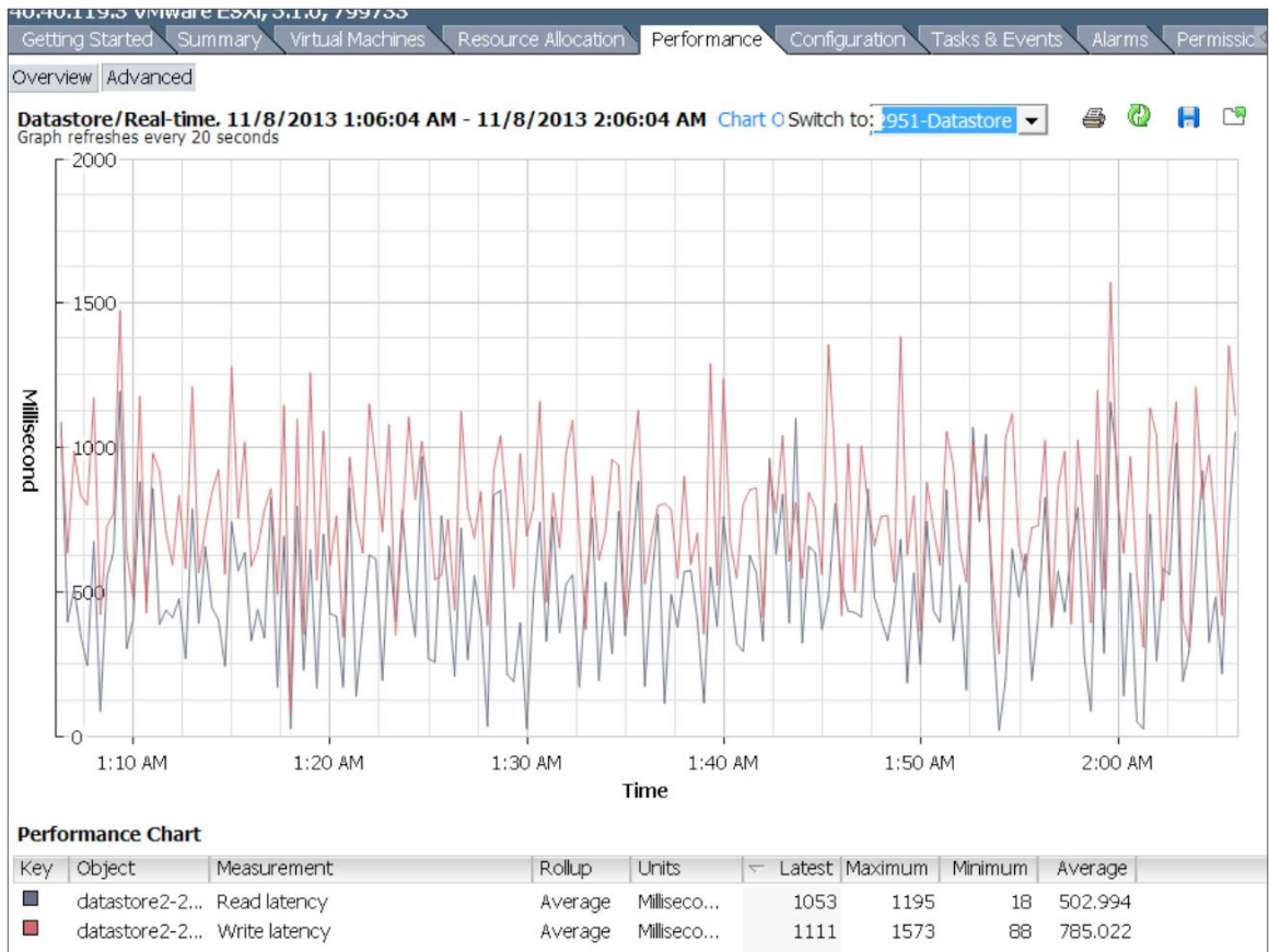
Figure 7. Read and Write Latency of the Cisco UCS E140D
