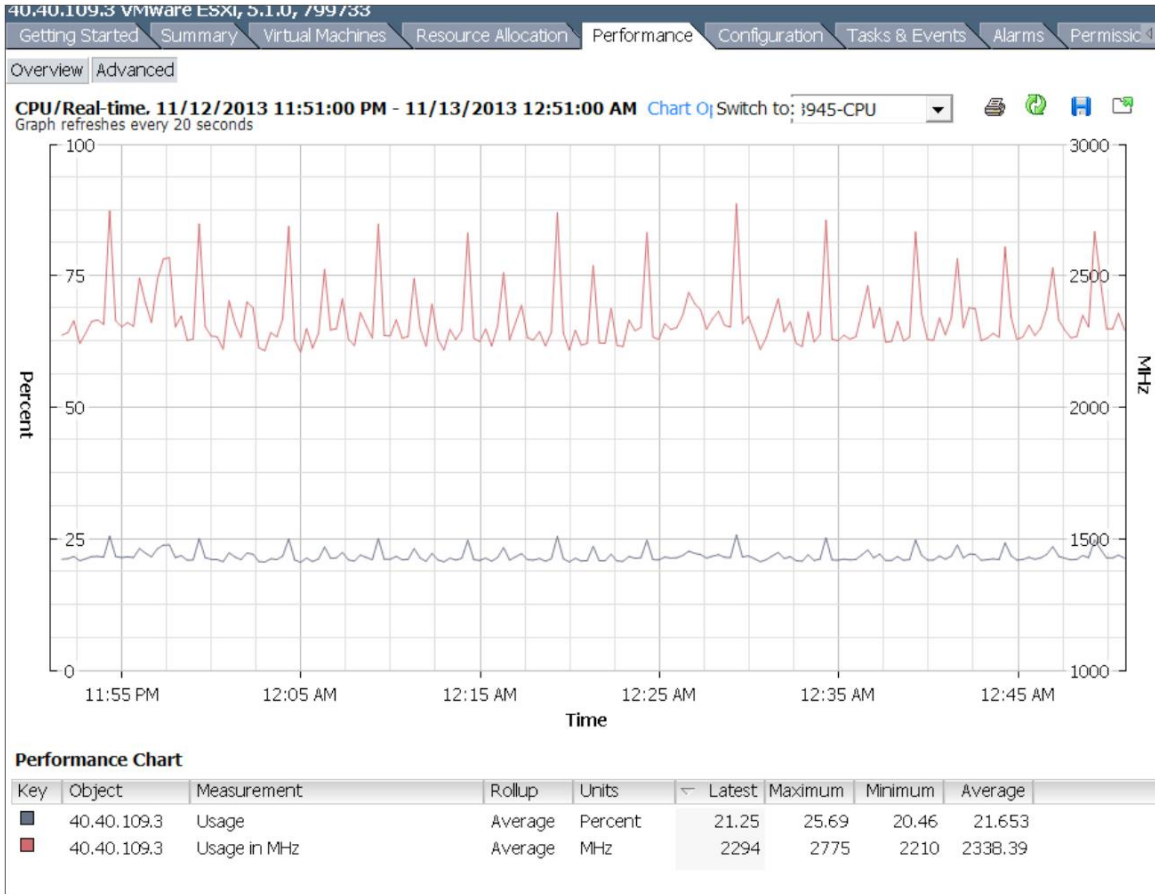
Figure 8. Overall CPU Utilization of the Cisco UCS E160D
