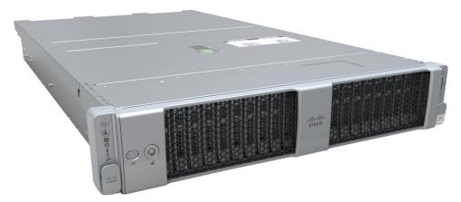
The Cisco UCS C245 M6 SFF Rack Server extends the capabilities of Cisco's Unified Computing System portfolio in a 2-Rack-Unit (RU) form factor with the addition of the AMD CPUs as well as 16 DIMM slots per CPU for 3200-MHz DDR4 DIMMs with individual DIMM capacity points up to 256 GB. The maximum memory capacity for 2 CPUs is 8 TB (for 32 x 256 GB DDR4 DIMMs1).
