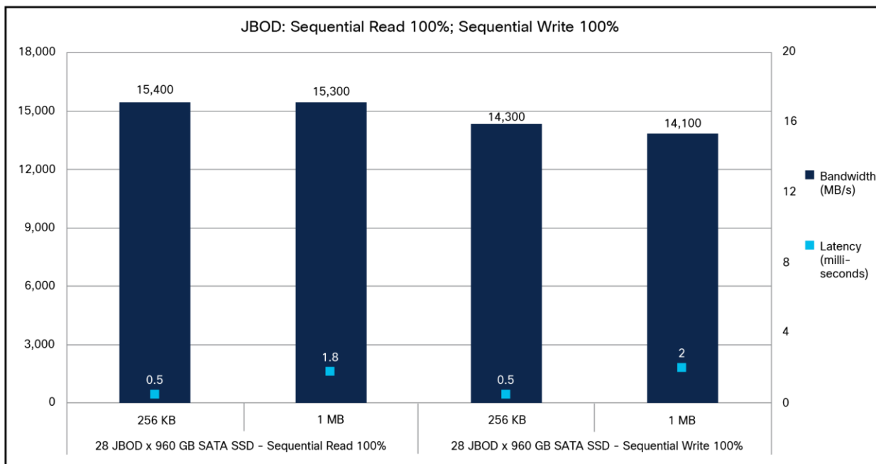
Figure 13. Cisco UCS C240 M7SX JBOD 100-percent sequential read; 100-percent sequential write
