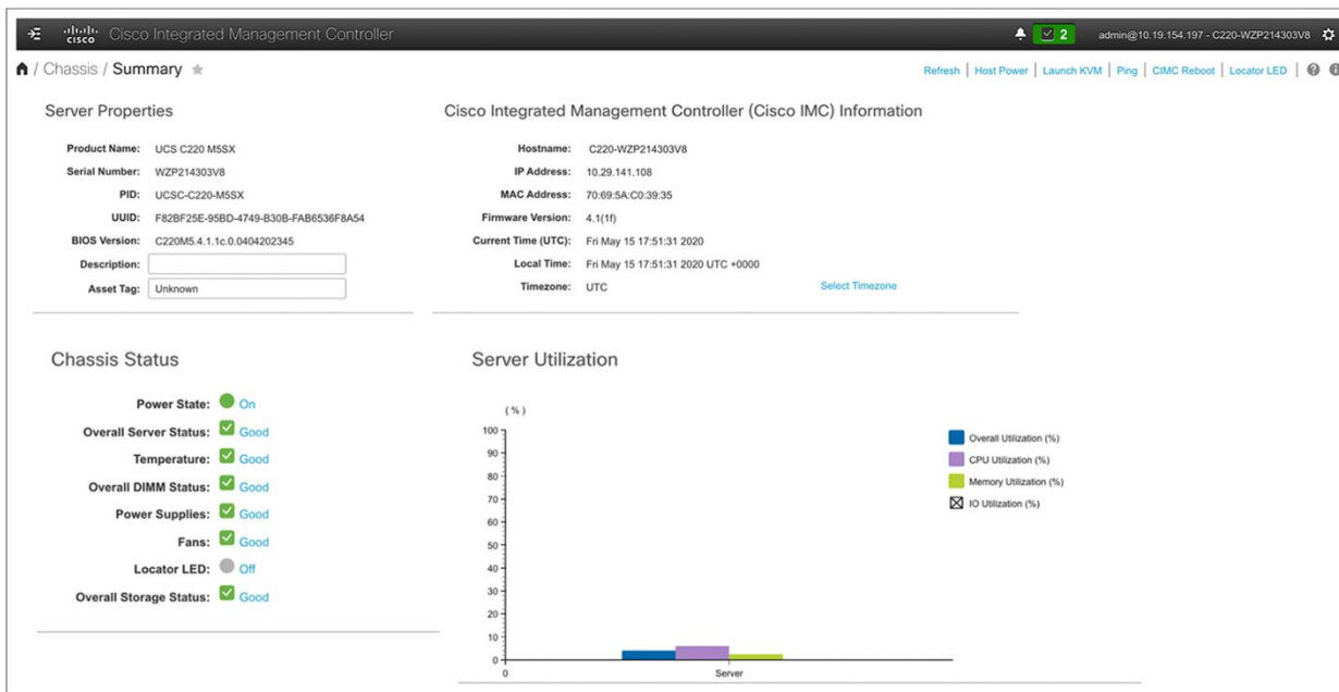
Figure 1. Cisco IMC server properties details, including chassis status and server utilization
