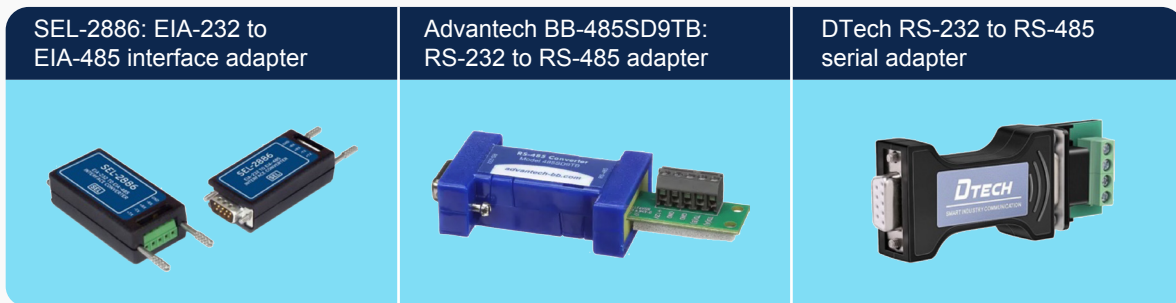
Figure 2. RS-232 to RS-485 adapters
