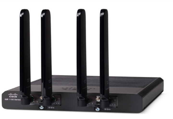
Figure 16. C1109-4PLTE2P front panel with two PIM slots
