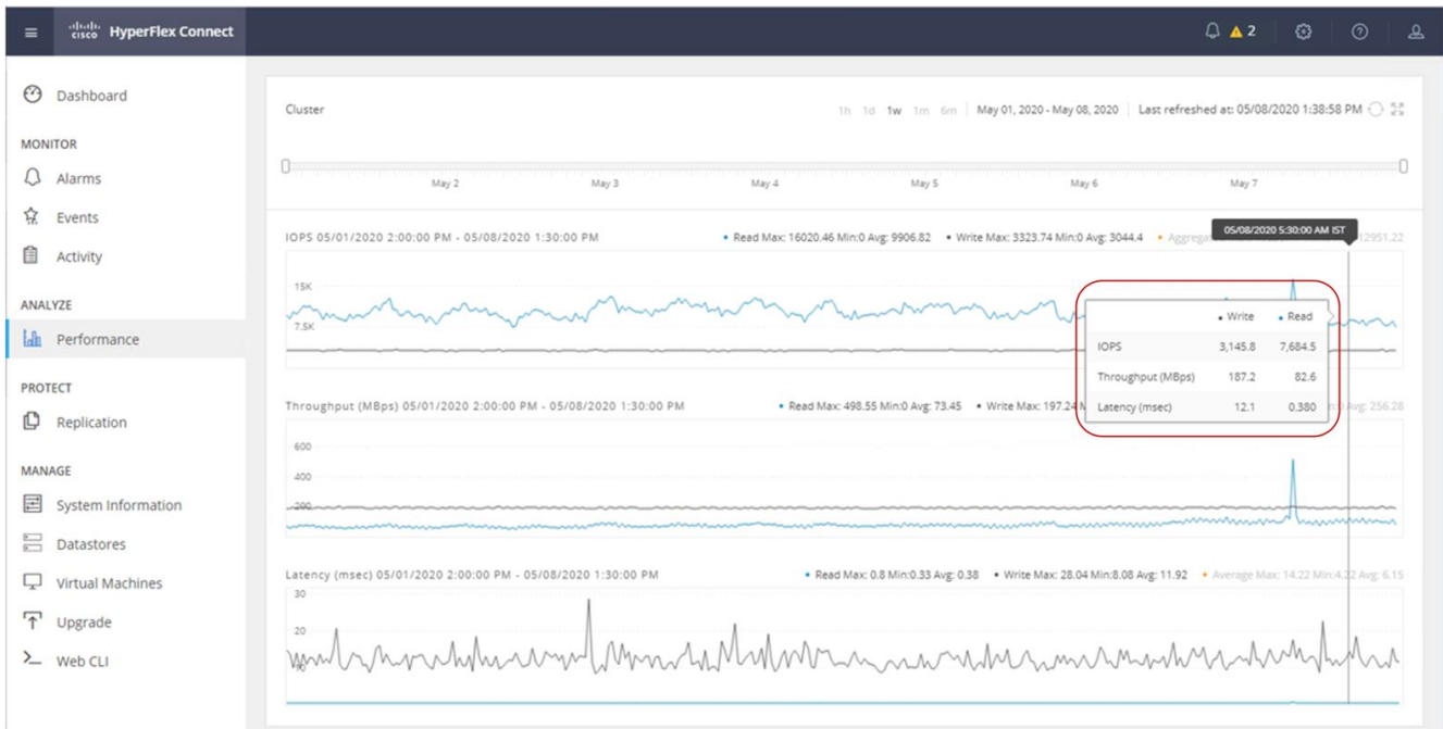
Figure 13. Average read-write throughput and latency of all recording servers observed in Cisco HyperFlex Connect
