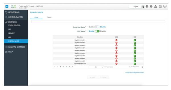
Energy saver Client mode will help in managing the end devices connected to the interface. Cisco EnergyWise uses a set of power levels to consistently manage power usage. The power level energy management settings available in Cisco Configuration Professional for Catalyst are Full, Hibernate, Shut, and Sleep.
