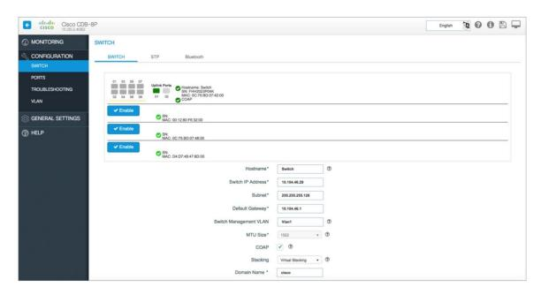
STP can be configured on the Configuration->Switch page. STP modes that are supported on Cisco Configuration Professional for Catalyst are RPVST, PVST, and MST. You can see details of VLAN ID, VLAN Name, Spanning Tree Status (enabled or disabled), and the bridge priority number.
