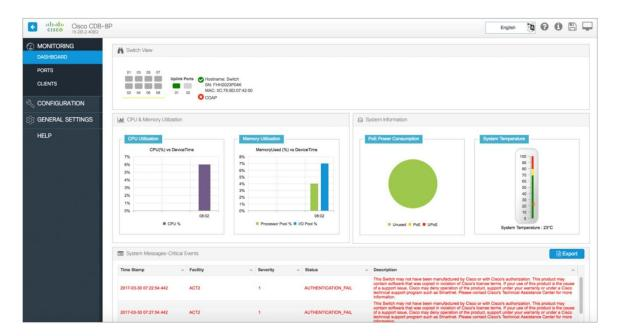
Ports monitoring enables users to track and monitor port parameters such as description, port status, and type. Details on a specific port in the table can be selected and highlighted by clicking on the port in the logical view at the top.
