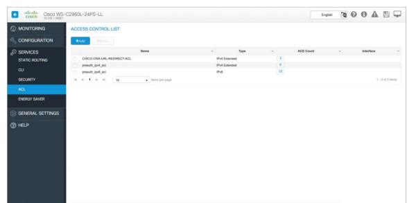
Customers can see the complete list of ACLs as well as the type of ACL and the ACE (access control entry) count.
