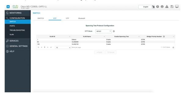
VTP is a newly introduced feature in Cisco Configuration Professional for Catalyst 1.4.0. VTP can be configured on the Configuration->Switch page.
