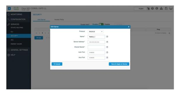
Access policy can be configured using Cisco Configuration Professional for Catalyst starting with the 1.4.0 release. Customers have the option to choose between 802.1X, Mac Authentication Bypass (MAB), and WebAuth. These policies can be applied to multiple interfaces at once. The default server groups are RADIUS and LDAP. Customers can choose from one of these server groups.
