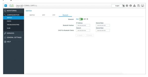
Starting with Cisco Configuration Professional for Catalyst 1.4.0, customers can configure switch virtual interfaces (SVIs) and assign IP addresses to the SVIs created. This can be done on the Configuration → VLAN tab.
