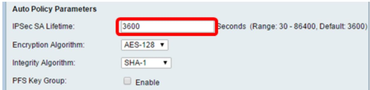
The screenshot shows the 'Auto Policy Parameters' configuration window. The 'IPsec SA Lifetime' field is highlighted with a red box and contains the value '3600'. The 'Encryption Algorithm' is set to 'AES-128', the 'Integrity Algorithm' is set to 'SHA-1', and the 'PFS Key Group' checkbox is unchecked.
