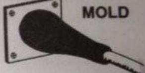
To apply - diagonally wrap a strip of Coax-Seal over a clean, dry connection making sure to overlap as you apply. Mold to form a smooth surface and to force out air.
