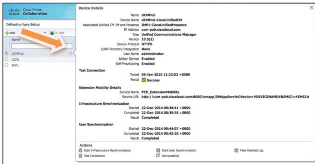
The screenshot shows the 'Device Details' page for the 'UCMPub' device. An orange arrow points to the 'Edit' icon in the 'Infrastructure Setup' table. The details include:
