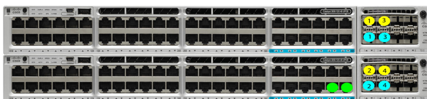
Dual 10/25GE ToR Switches (standalone or stacked)
