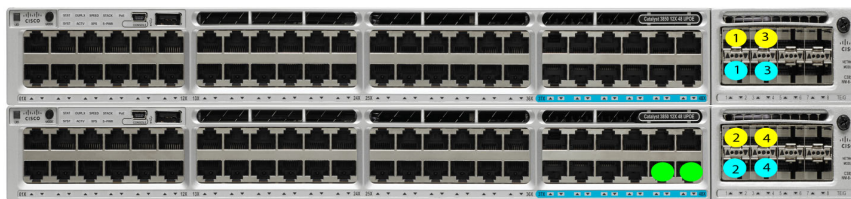
Dual 10/25GE ToR Switches (standalone or stacked)
