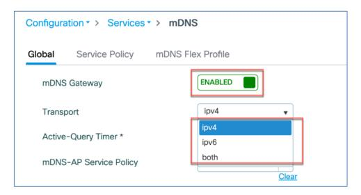
In Local Bridging mode (when mDNS GW is not enabled), packets with mDNS multicast IP and multicast mac will be sent on multicast CAPWAP tunnel. A multicast CAPWAP tunnel is a special CAPWAP tunnel used for reducing the number of copies of multicast packet that are required to be generated for each AP CAPWAP tunnel. Sending packets on the multicast CAPWAP tunnel requires the outer IP header to be destined to the multicast CAPWAP tunnel's address, which all APs are subscribed to.
