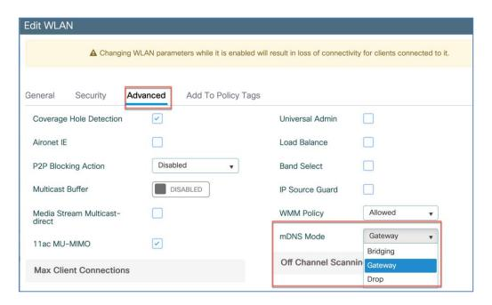
mDNS Gateway when enabled on the controller has a proxy function that is primarily used to reduce the multicast on the "AIR" interface; with many new devices adopting mDNS as a service discovery mechanism it becomes imperative to support it so that the AIR interface could be effectively used. In Flex mode the caching services will be performed on the FC AP itself.
