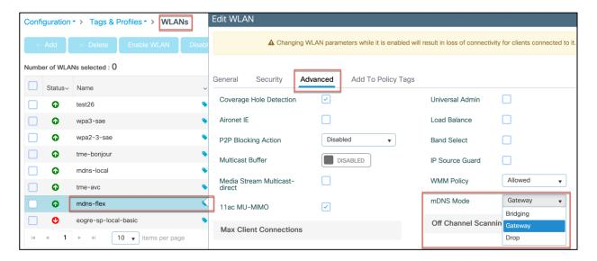
The following command under Configuration > WLAN, will Map the Policy Profile to the WLAN with mDNS GW mode enabled in the previous step. Previously configured Policy Profile and Policy Tag will be added to the selected WLAN.
