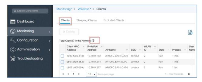
When the **GW** is enabled on the Global and WLAN level— then both wired and wireless services being cached on the controller. In setup as shown below there are 3 Wireless and 1Wired Apple TV connected.
