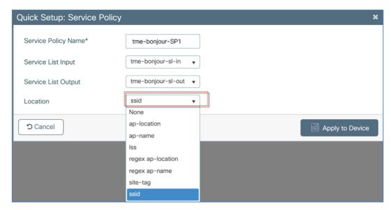
**Based on AP Name selected:** There are use cases where the requirement is to only respond with mDNS services which are learned from the same AP as that of the querying client. In release 17.1 mDNS location-based filtering is enhanced to filter services from the same AP-name if configured.
