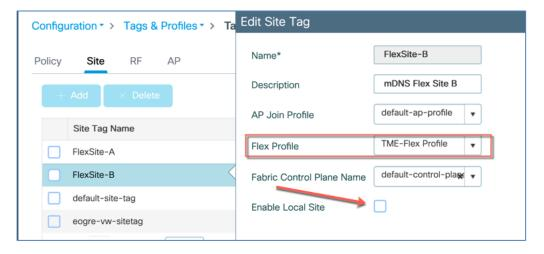
In the next step under the Configuration>Tags&Profiles>Tags choose the "AP>Static" tab choose an AP and map to that AP(s) with Policy Tag Name or WLAN "bonjour-tme" and the Site Tag Name "FlexSite-A" created in the steps above and as shown in the example screen shot below.
