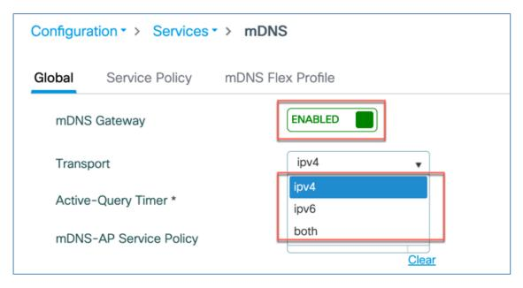
When mDNS gateway is enabled, mDNS packets will be consumed by the mDNS gateway and clients or device will be deprived of learning this service. In-order to share the service with the device and to provide ease of configuration to the administrator, few standard Service Types will be shared by **default** on the wireless network. The list comprising of these standard service types is termed as Default Service Policy and would have the following service types as listed in the table below.
