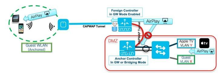
Begin with release 17.1, Wired Guest support was added in C9800 controllers. The new mDNS enhancement added support for wired guests as illustrated below. mDNS support for wired guest is now on par with the wireless clients.
