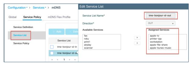
The Service list is matched on IN (request, ingress filter) and/or OUT (respond, egress filter) to the queries. The list shown comprising of the service types is termed as Master Service List and is not a part of the Default Service List.
