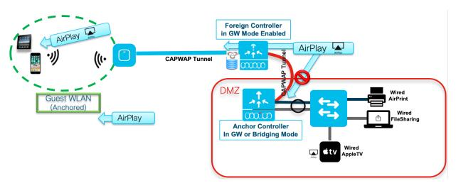
As part of this new enhancement in rel 17.1 new guest-lan profile specific CLI/WebUI is added to allow the administrator to configure mDNS mode on the guest-lan profile. This will be same CLI/WebUI configuration as what is present currently in WLAN profile mode for setting the mDNS mode. The default mDNS mode on the guest lan (without any explicit configuration) will be mDNS Bridging mode.
