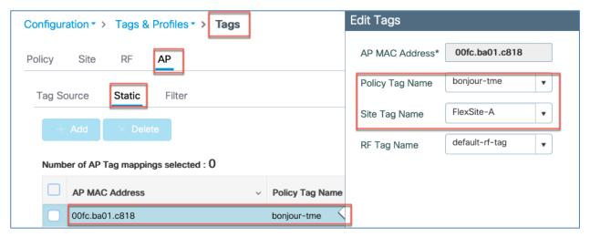
By applying the above-mentioned Site Tag with "Enable Local Site" unchecked the AP(s) will be converted to the Flex mode and all Flex policies and profiles will be applied to them. Verify that all selected Tags and Policies are applied correctly by going to Configuration>Wireless>Access Points and selecting AP(s) to which the Tags were applied.
