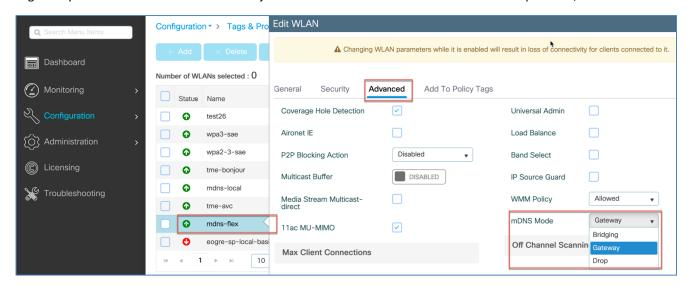
In the release 17.3 new Flex Mode mDNS configuration steps available to configure the mDNS Flex Profile under the mDNS configuration tab.
