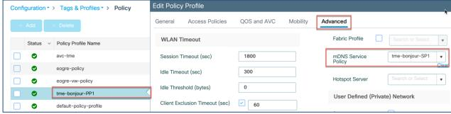
WLAN mDNS Mode is configured under WLAN tab. Different WLANs can have different Policies and Profiles, which can be also AAA overridden for more granularity.
