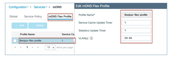
After the mDNS Flex profile is configured, configure the other parameters in that section and the Supported Local VLANs.
