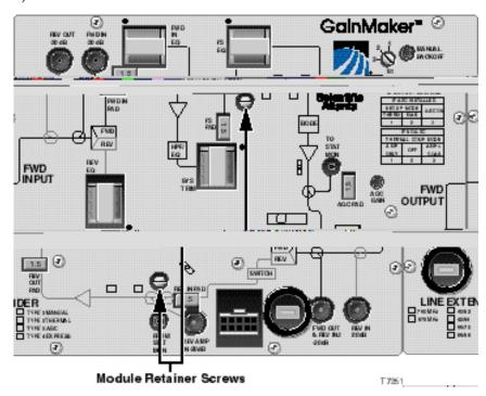
4. Plug the 10-pin keyed connector of the power supply cable into the amplifier module.
