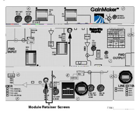
6. Depending on the type of amplifier cover screws on the amplifier module cover, use either a Phillips-head or T-15 Torx bit screwdriver to loosen the 12 screws, then remove the cover.
