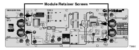
6. Place the amplifier module upside down on a secure surface.
