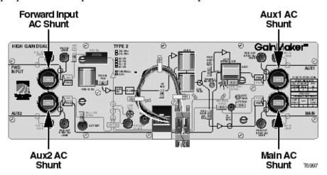
**Result:** Power is reconnected to the system amplifier.
