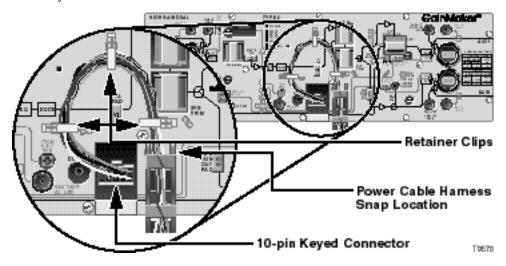
4. Route the power cable through the white plastic retainer clips.
