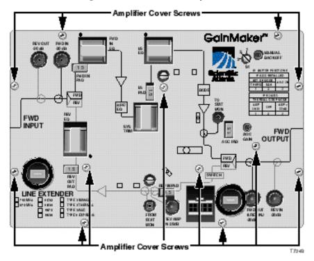
7. Remove the amplifier module from its housing, and place the amplifier module on a secure surface.
