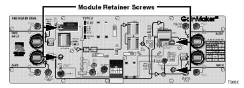
3. Plug the 10-pin keyed connector of the power supply cable into the amplifier module.
