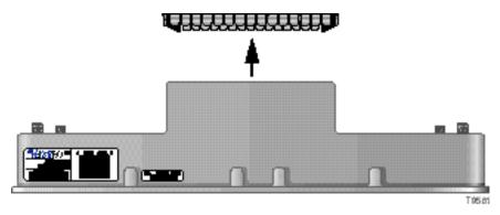
2. Carefully pull straight up on the reverse switch to remove it.
