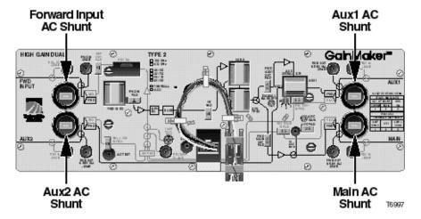
**Result:** Power is disconnected from the system amplifier.
