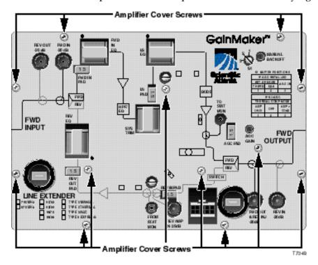
3. Using a flat-head screwdriver, secure the amplifier module to the housing by tightening the two module retainer screws from 6 in-lb to 9 in-lb (0.7 Nm to 1.0 Nm).
