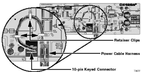
3. Remove the power cable from the white plastic retainer clips.
