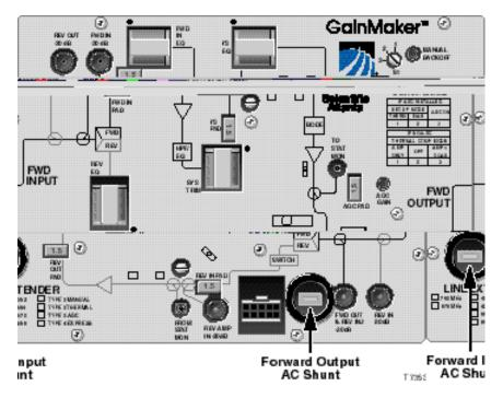
**Result:** Power is disconnected from the line extender.
