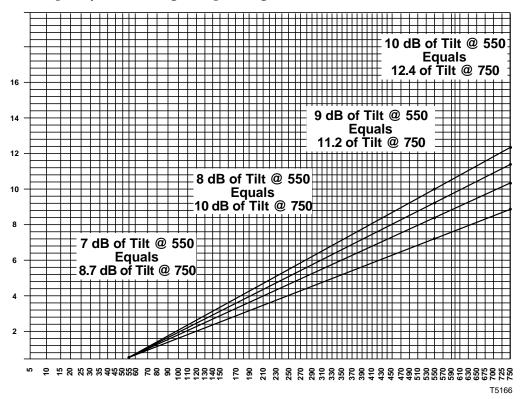
For example: If the amplifier operating levels are 42 dBmV with an operating tilt of 10 dB at 750 MHz, the operating level at the pilot frequency of 445.25 MHz would be 39 dBmV. This was found by taking the difference in tilt between 750 MHz and 445.25 MHz (10-7=3 dB). Then subtract the difference in tilt from the operating level (42-3=39 dBmV).
