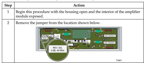
Install the correct fixed reverse equalizer for your system as specified by the design print in the reverse equalizer slot.
