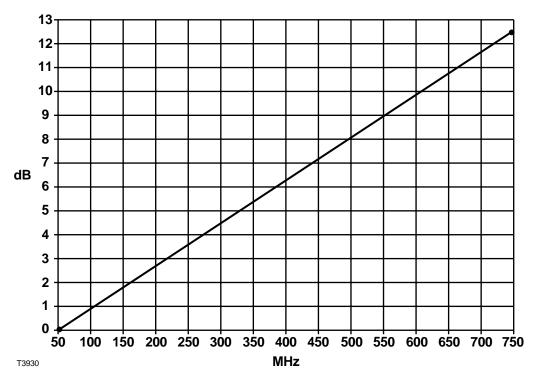
For example: If the amplifier's 750 MHz output level is 46 dBmV with a linear operating tilt of 12.5 dB (from 50 to 750 MHz), the corresponding output level at 550 MHz would be 42.5 dBmV. This was found by taking the difference in tilt between 750 and 550 MHz (12.5 - 9 = 3.5 dB). Then subtract the difference in tilt from the operating level (46 - 3.5 = 42.5 dB).
