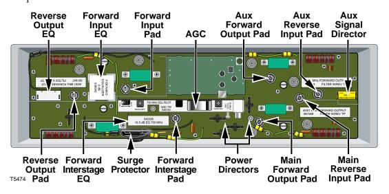
750 MHz System Amplifier III Types 1 and 2 Installation and Operation Guide
