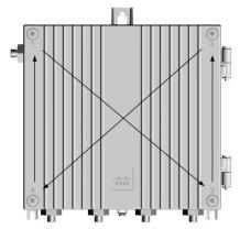
The pin length of the PG 11 cable connector at input and output is shown on the cover plate of the amplifier. If needed, trim the connector with a wire cutter.
