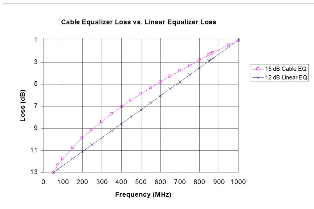
As shown above, both the linear equalizer and the cable equalizer introduce greater signal loss at lower frequencies. However, whereas the cable equalizer response is curved, the linear equalizer response is a straight line, indicating equal loss per unit of frequency.
