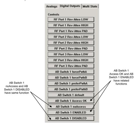
To change the preferred path of AB Switch 1, you must select both **AB Switch 1 Access OK** and **Switch 1 Enabled**. These controls work together like a pair of deadbolt locks: both must be "drawn" to enable the preferPathA and preferPathB controls.
