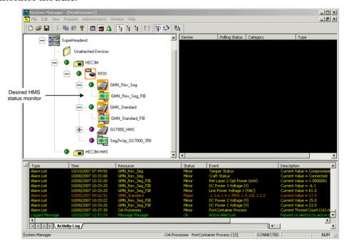
2 Right-click on the status monitor and select **Data Display**. The Data Display window opens as shown below.
