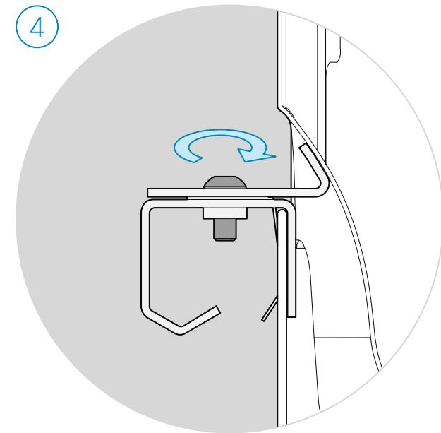
Tighten the screws and check that the clamp is securely fastened.
