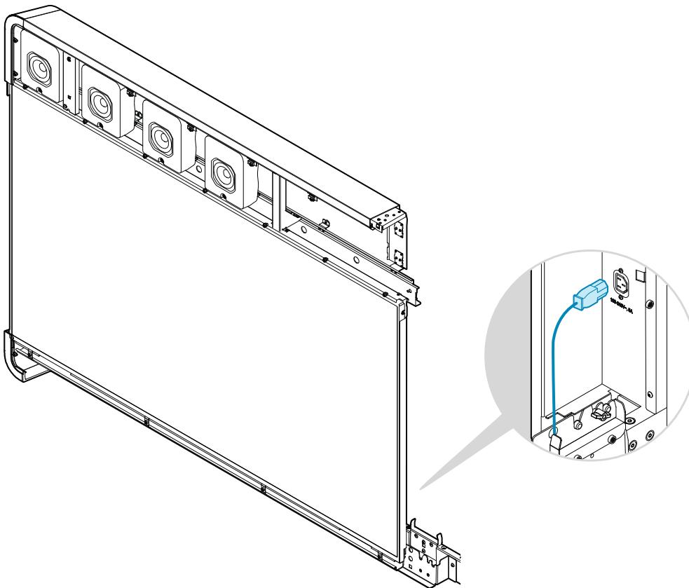
A power cable is attached to the right side of the screen. Connect it to the nearby connector.
