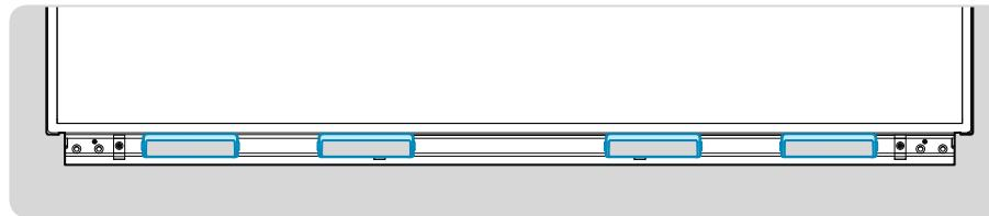
Four people must work together to mount the screen. At least two people should lift the screen using the lifting handles. The other people must help stabilizing the screen and check that it enters the slots properly.
