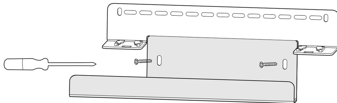
Due to the variety of wall constructions, the installer has to bring the parts that are required to fix the wall mount brackets securely to the wall.
