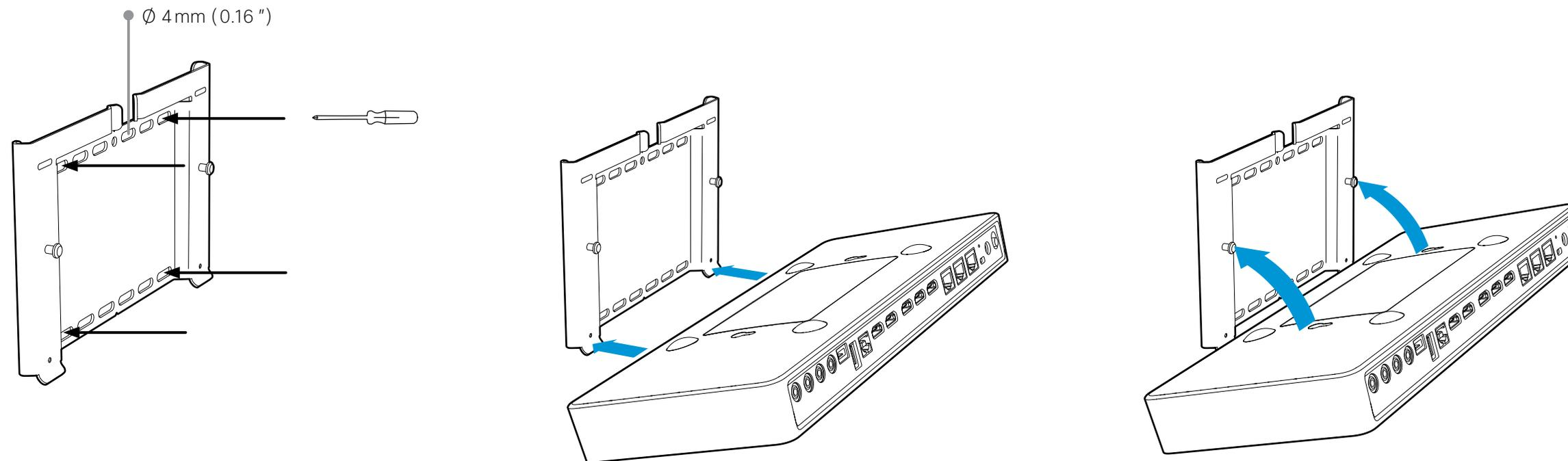
Use four screws to fasten the bracket to the wall.
