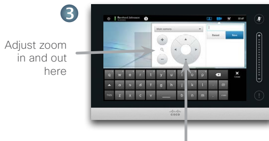
Use these controls to define the direction in which the camera shall point (also known as Pan control).
