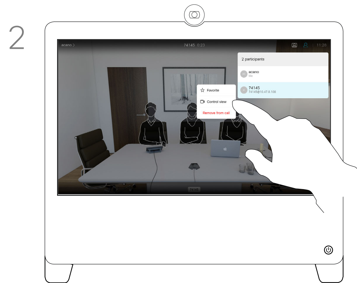
Tap the participant, whose camera you want to control, then tap Control view .
