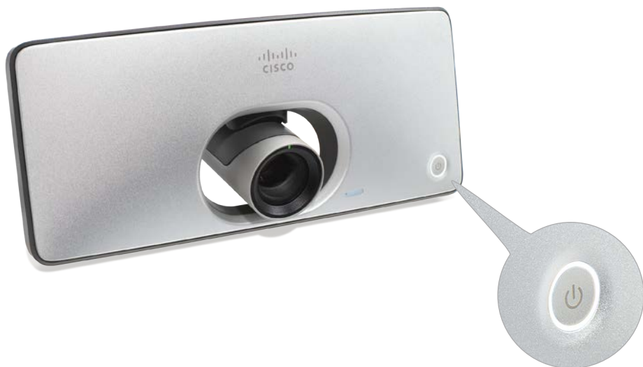
Power button with LEDs encircling the button
