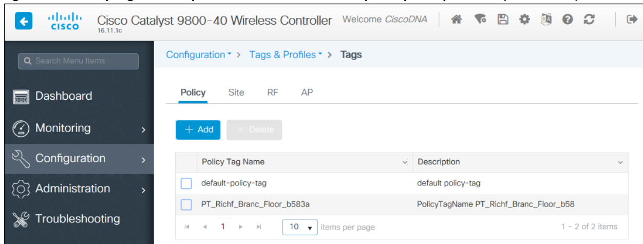
Figure 75 Policy Tag created by Cisco DNA Center within the primary enterprise WLC (WLC-9800-1)
