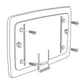
2 Align the two slots on the underside of the router chassis to the notches in the mounting plate. Then gently slide the router chassis down onto the notches.
