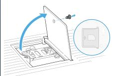
2 Slide the SIM card holder cover towards the socket cover hinge and open it.
