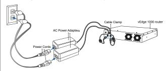
• Caution: If you are connecting AC power to the router, it is recommended that the building have an external surge protective device installed.
