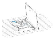
4 Close the SIM card holder cover. Then close the socket cover and screw it shut.
