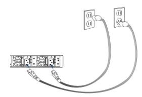
① Caution: If you are connecting AC power to the router, it is recommended that the building have an external surge protective device installed.
