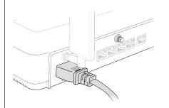
Caution: If you are connecting AC power to the router, it is recommended that the building have an external surge protective device installed.
