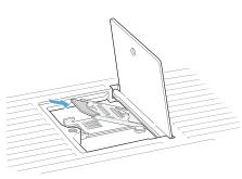
4 Close the SIM card holder cover. Then close the socket cover and screw it shut.
