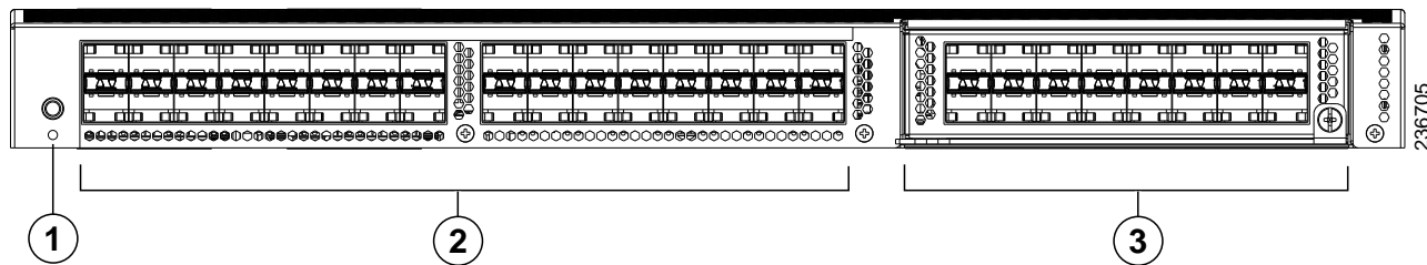
Figure 6 48-port Fabric Interconnect Chassis Detailed Rear View
