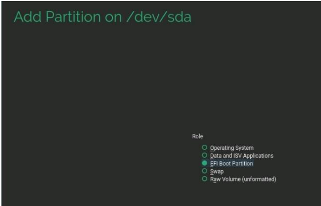
Figure 31. Adding a partition: Specifying the role
