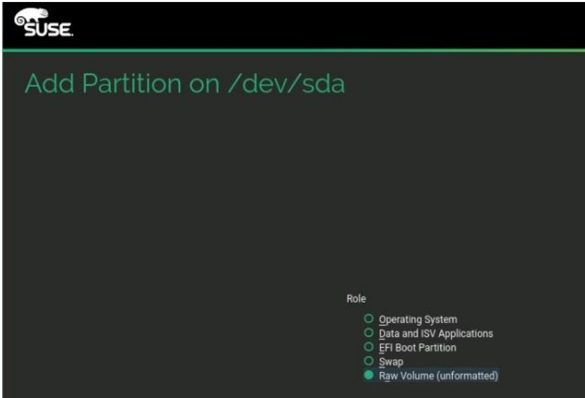
Figure 34. Adding a partition: Specifying the role
